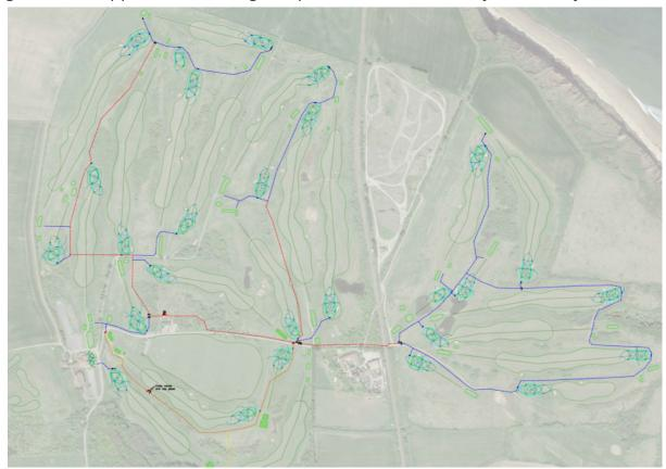
The map above shows where pipework will be run, with red and blue showing the mainline. The bottom section in orange has already been completed and our aim is to do the seven greens above the public bridleway seen in the top left of this image.
